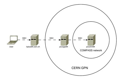
Figure 4.2: A depiction of how computers in the internal COMPASS network can be accessed from outside of the CERN GPN
