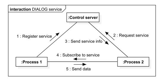
Figure 1.5: The concept of network communication using services in DIALOG
