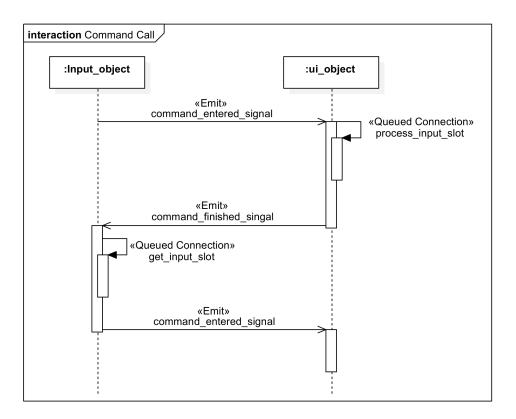
Figure 6.2: Signal-slot structure of a command call
