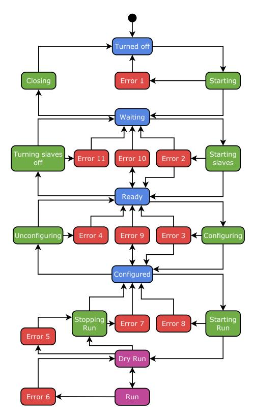
Figure 1.4: The state machine diagram of the Master process [16]
