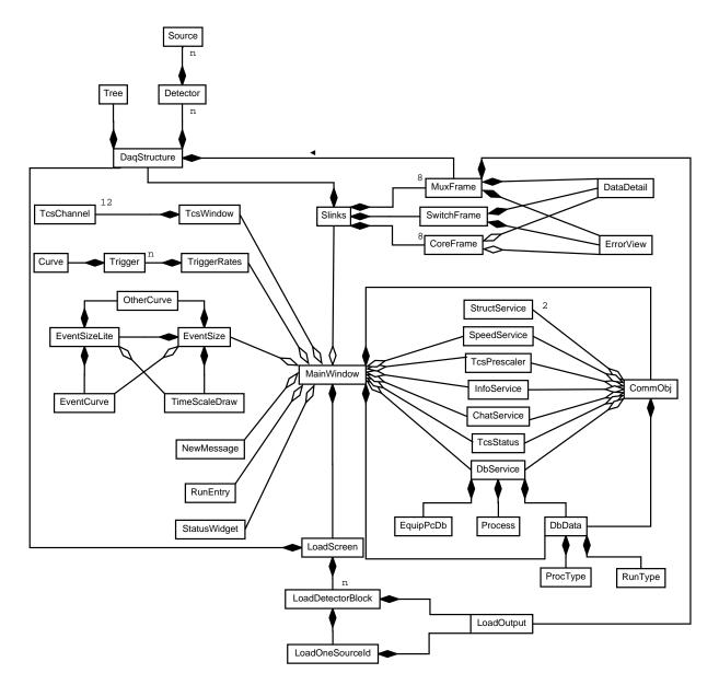
Figure 4.1: UML class diagram of the GUI. Not included: low-level classes used for registry representation and message encapsulation. Cf. section 1.5.2 of [16] for more information.
