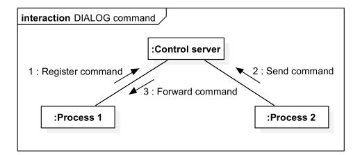
Figure 1.6: The concept of network communication using commands in DIALOG
