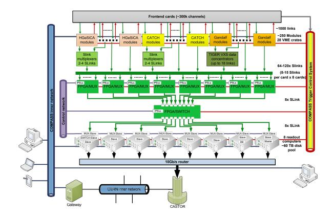
Figure 1.2: Hardware structure of the DAQ [11]
