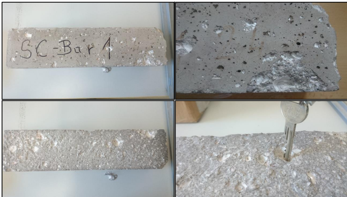
Figure 40: Damage of barite aggregate concrete after heating to 400°C
