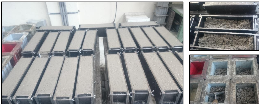
Figure 18: Samples preparation – example of one out of the five sets – Barite concrete
