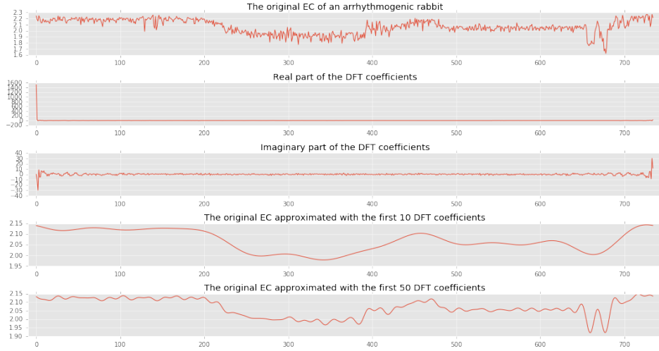
Figure 2.28: The example of DWT coefficients and of EC reconstruction using DFT coefficients. From top to bottom: original EC, real part and then imaginary part of DFT coefficients, EC reconstruction with the first 10 and the first 50 DFT coefficients.
