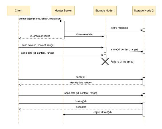
Figure 3.2: Diagram of an example situation of a write of an object with replication factor 2 with failure of one of the nodes
