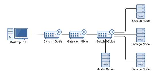
Figure 5.1: Diagram of the network connection configuration of the computers used during the testing
