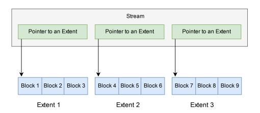
Figure 2.3: Structure of a Stream stored on the Stream Layer of Windows Azure Storage
