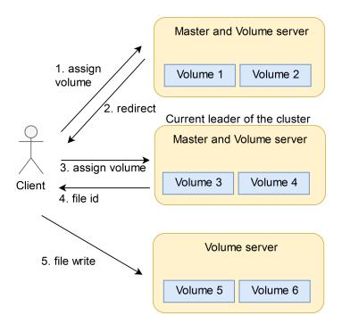
Figure 2.4: Diagram of align assignment of a volume and file ids for write by current leading master server
