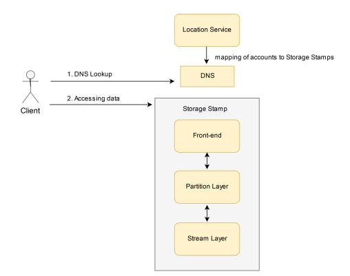
Figure 2.2: Schema of high-level architekture of Windows Azure Storage
