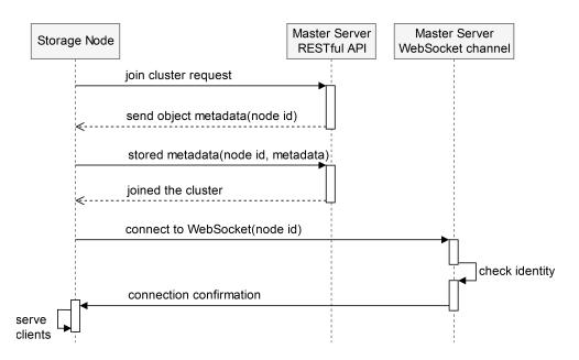
Figure 3.9: Protocol of the communication during the connection of a node to the cluster
