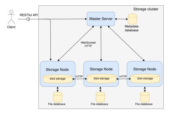
Figure 3.1: Diagram of designed architecture of the storage cluster with communication channels between components
