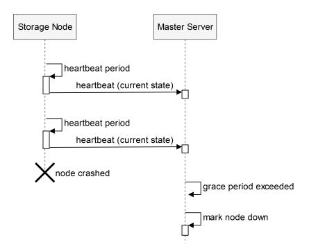
Figure 3.10: Sequence diagram of heartbeats sent from a storage node to the master server
