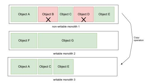
Figure 3.8: Process of compaction of a monolith and selection of a new location for the living objects
