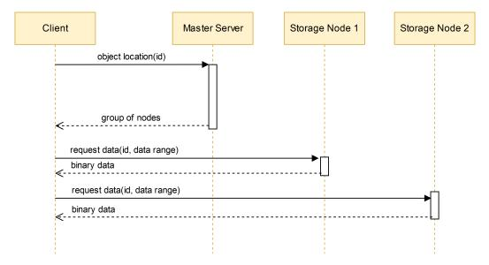
Figure 3.3: Diagram of sequence of client requests necessary for retrieval of object data
