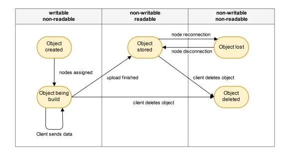
Figure 3.5: Diagram of the main states of an object and the transitions between them
