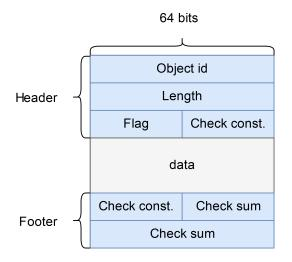
Figure 3.7: Diagram of the structure of an object stored in a single monolith file
