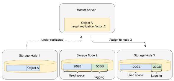
Figure 3.11: Diagram of the strategy for assignment of an under replicated object to a storage node
