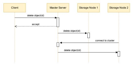
Figure 3.4: Process of asynchronous object deletion after client request
