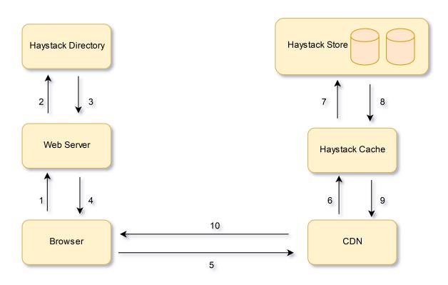
Figure 2.1: Schema of a sequence of requests necessary for retrieval of an image from the Haystack store
