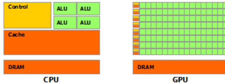
Figure 2.3: The GPU Devotes More Transistors to Data Processing [2]
