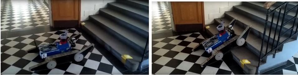
**Figure 6.20:** Test drive up the stairs
