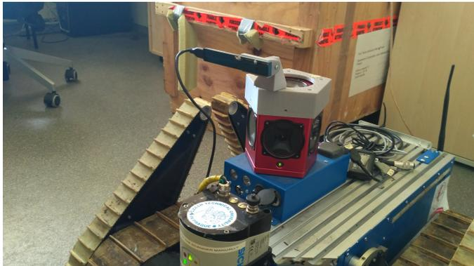
Figure 5.1: RealSense mount
