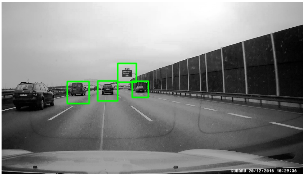
Figure 3.4: Image after the histogram equalization and grayscale conversion. The green rectangles are objects of interest recognized by Viola-Jones detection framework. Notice the false alarm in the center and undetected car to the left.
