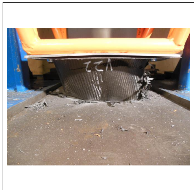
Figure 4: Attenuator after Impact
