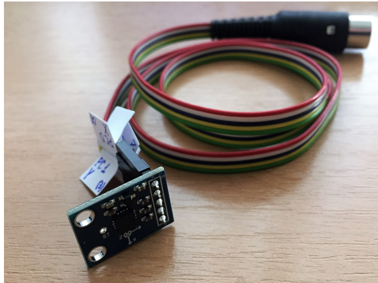
Figure 4.2: Analogue MEMS 3-axis accelerometer ADXL335.
