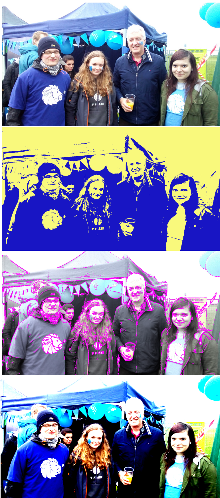
Figure 20. Implemented low-vision filters: original image, Otsu threshold, Sobel edges, high contrast
