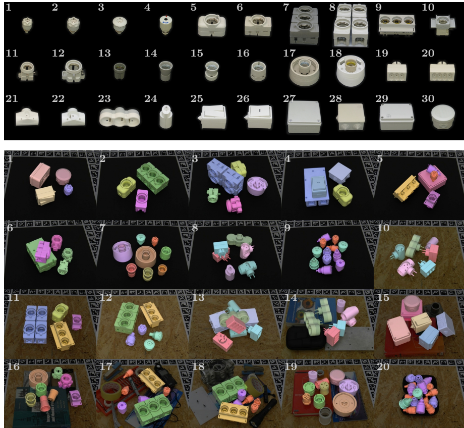
Figure 5.1: T-LESS includes training images and 3D models of 30 objects (top) and test images of 20 scenes (bottom). The shown test images are overlaid with colored renderings of 3D object models at the ground truth poses.
