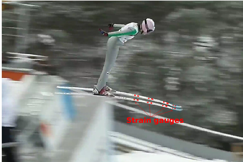
Figure 1: Application of strain gauges to measure the stress applied on the ski during ski jumping.
