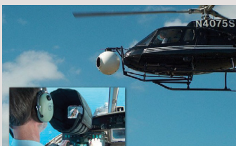
Airborne surveying applications use KVH's DSP-3100 to provide the stabilisation necessary to produce clear images.
