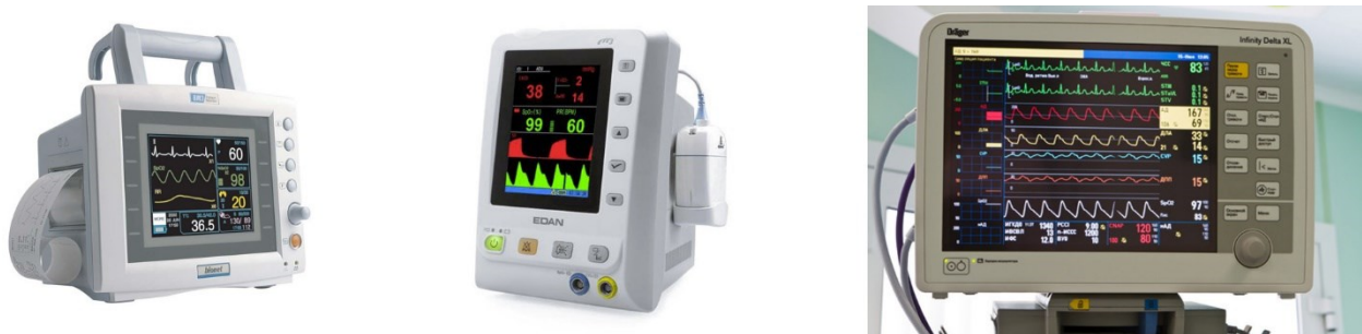
Figure 43 Different types of patient monitors with different way how to show curves on their screens [77], [78], [79]
