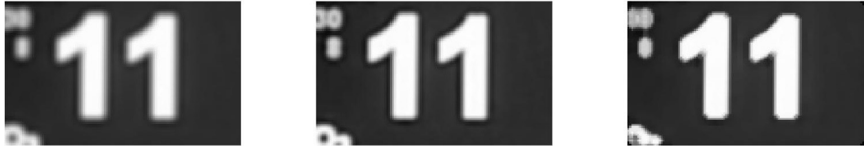
Figure 24 Region of interest after applying filters with kernel 5x5 px. Gaussian; average; median
