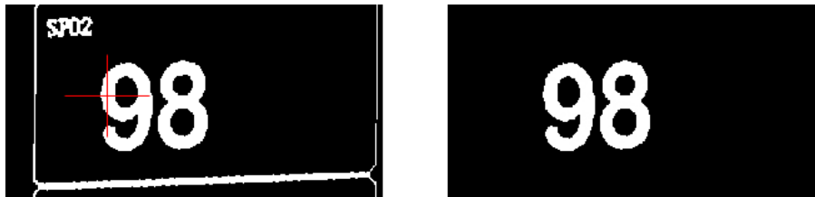
Figure 11 Manual selection of the digit; areas filtered only on appropriate candidates in the distance from selected digit [80]
