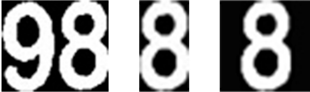
Figure 35 region of interest in bounding box; one separated candidate for digit; one candidate resize to 35x35 px with the same aspect ratio as original
