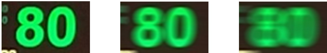
Figure 58 Captured digit in static scene; Captured digit during gently moving with patient monitor or camera; Captured digit during quick moving with patient monitor or camera
