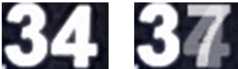
Figure 33 Candidates for digits obtained correctly; candidates for digits obtained incorrectly between two values
