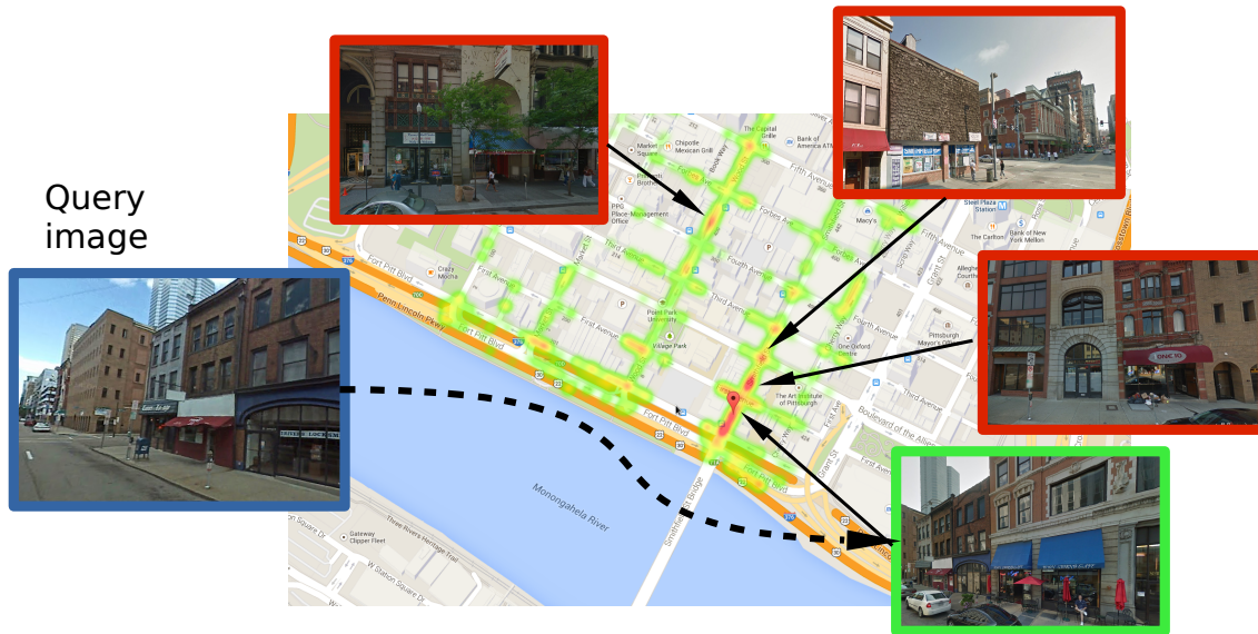
Figure 1.2: Place recognition by per-location classifiers. At each place on the map we train per-location classifier. The classifier learns relative importance of the image features for recognizing certain location. Given the unknown query image (blue frame), the similarity with the database images is measured by the calibrated classification score. The heat map layer indicates distribution of the calibrated classification score for the given query image. The four top-ranked database images are shown with its respective location in the map. Notice that one retrieved image is correct (green frame) and depicts the same place while other three top-ranked are incorrect (red frame).
