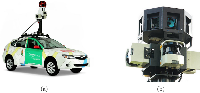
Figure 3.1: Google Street View capturing equipment. (a) A Google car with capturing equipment. (b) Detail of the capturing equipment. The Street View capturing device contains a spherical camera system, LiDAR, inertial measurement unit (IMU), accurate GPS, WiFi monitor and pollutant sensors.
