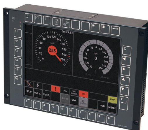
Technical and diagnostical display [AMiT Transportation]
