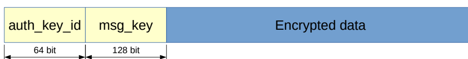
Figure 3.3: Expected form of sniffed data where 64-bits of key fingerprint are followed by msg_key and encrypted data.
