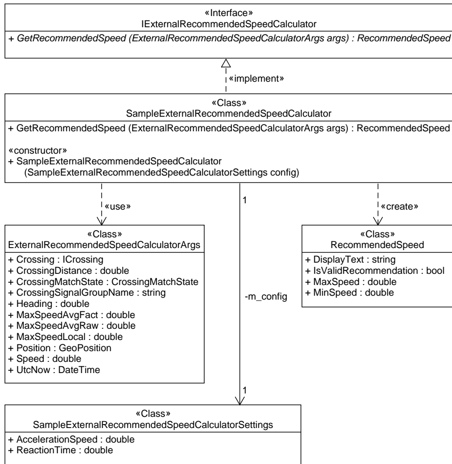
Figure 6.1: UML Class Diagram of Speed Calculation Component
