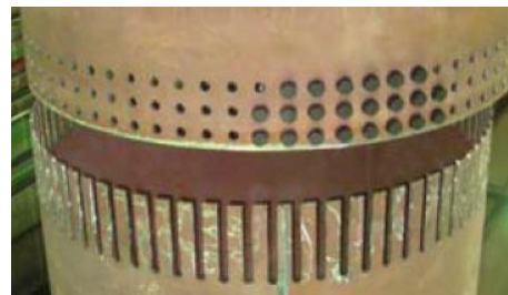
Friction connection (HISTWIN project)
