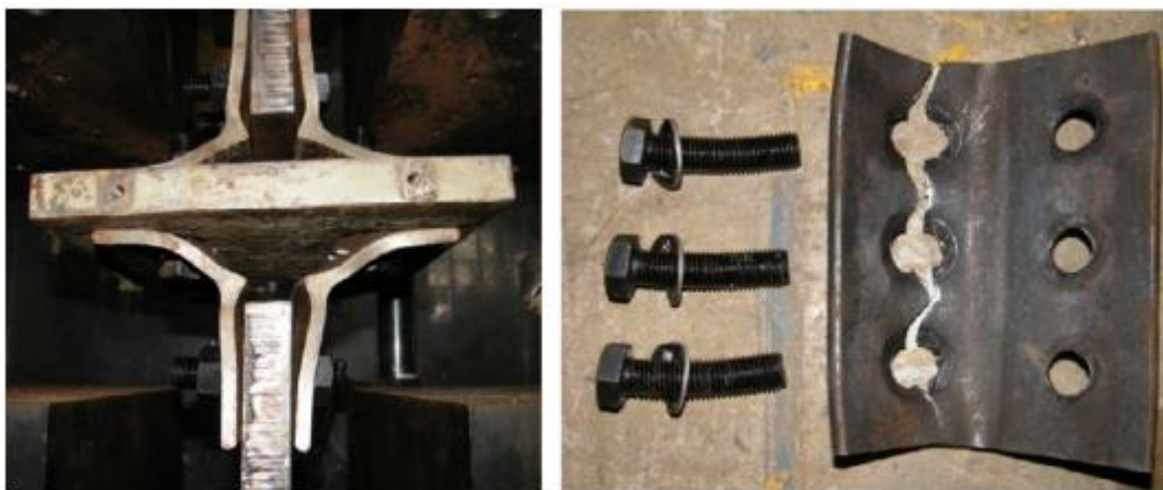
Figure 14. Angle fracture close to heel (A90-9-60-III).
