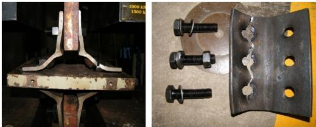
Figure 13. Angle fracture at bolt holes (A90-8-50-I)
