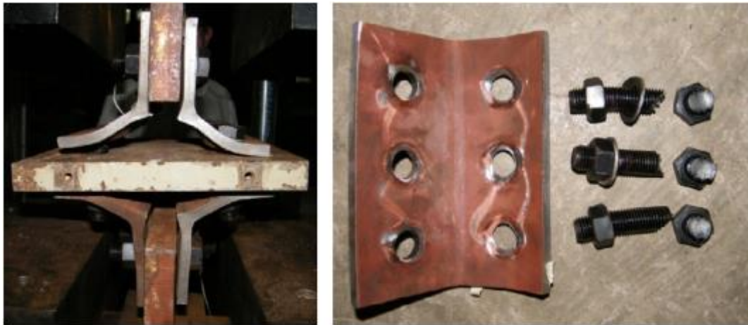
Figure 17. Bolt fracture with yielded angles (A90-10-50-IV).
