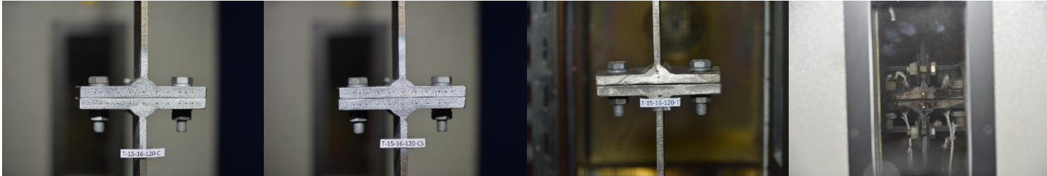
Figure 46. T-Stubs before experiment for T-15-16-120
