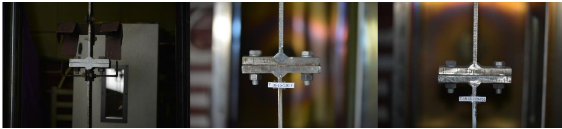
Figure 52. T-Stubs before experiment for T-18-16-120
