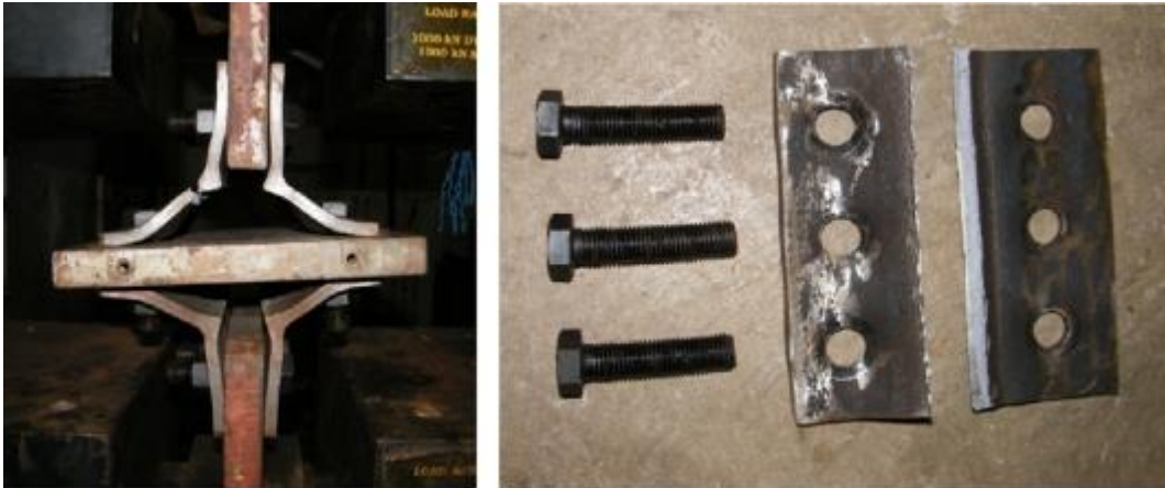
Figure 14. Angle fracture close to heel (A90-9-60-III).
