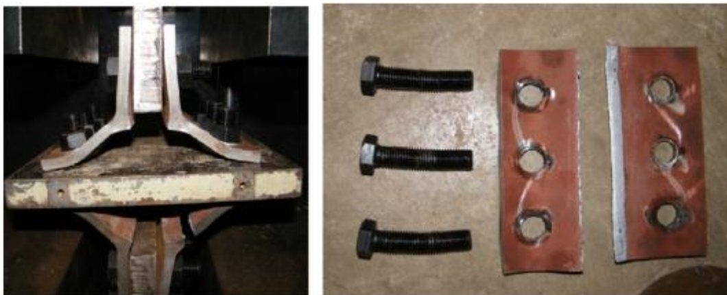
Figure 16. Angle fracture close to heel with yielded bolts (A90-10-60-IV).
