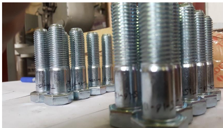
Figure 39. Bolt class 10.9 measured and marked
