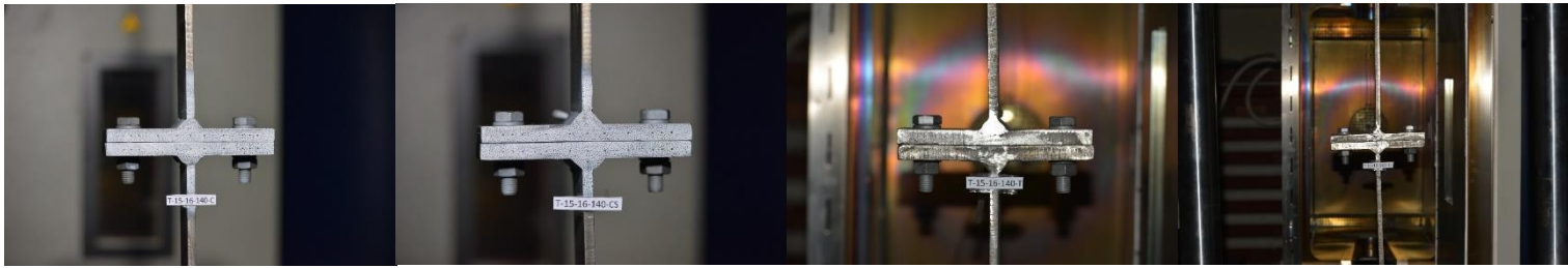
Figure 49. T-Stubs before experiment for T-15-16-140
