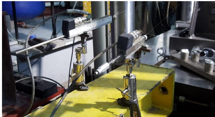
Figure 36. Rod type position sensors from novotechnik
