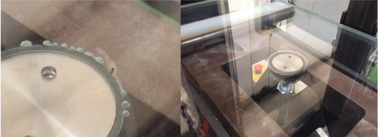
Figure 4.22 Origin and the propagation of glass-foil delamination
