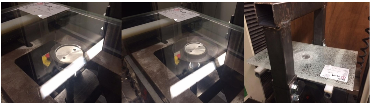
Figure 4.19 Spreading delamination and brittle failure (F1-01)
