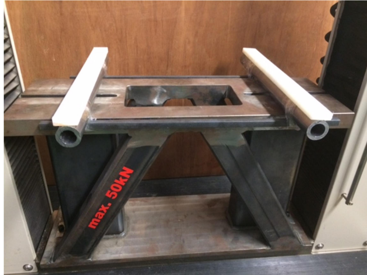
Figure 4.17 A steel bed with cylindrical supports and plastic washers
