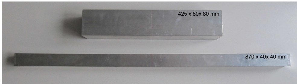
Figure 5.6: Metal prisms used for NF RCS measurements.
