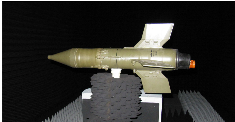
Figure D.7: Image of 9M14 Malyutka missile in anechoic chamber.
