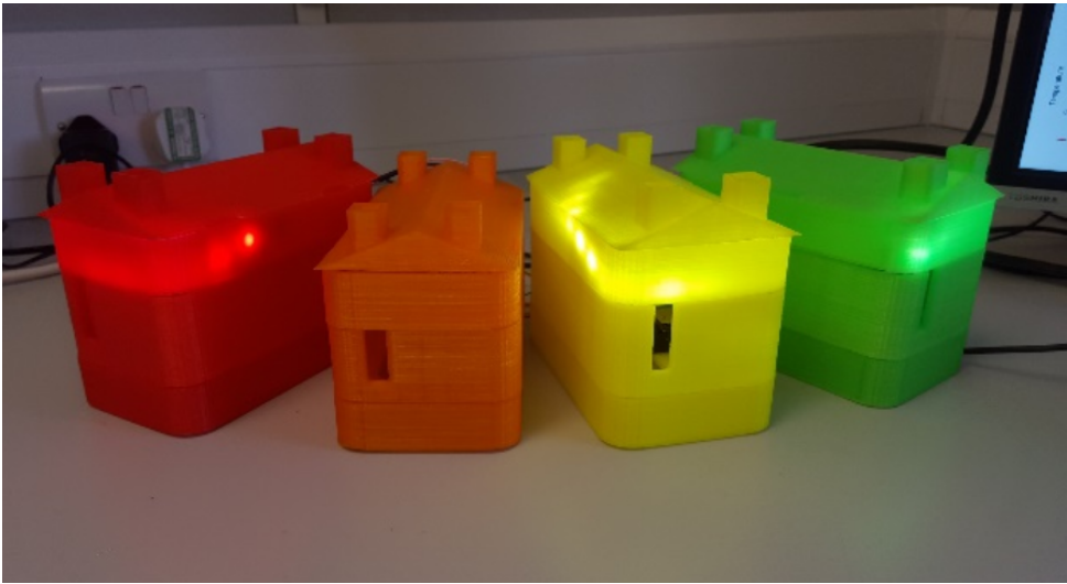
Figure 5.17: 3D printed houses used for smart-metering demonstration.
