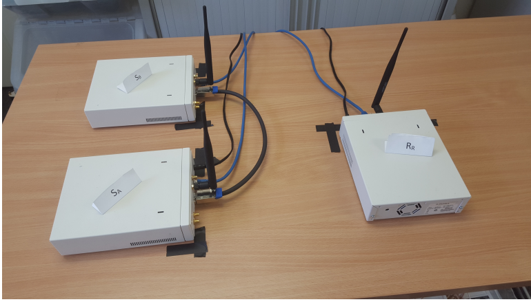
Figure 6.33: Compact laboratory placement of the network nodes for the CIP verification experiment.
