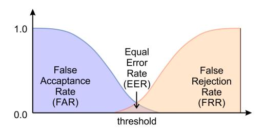
Figure 3.2: In this figure we can see the relation between the False Acceptance Rate the False Rejection Rate and the Equal Error Rate (adapted from http://goo.gl/VZ2U9z).
