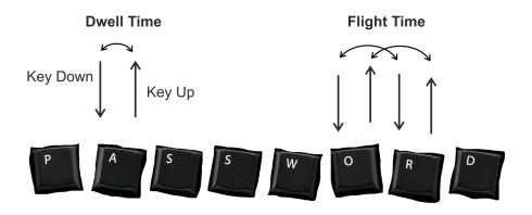
Figure 3.1: In this image we can see the Dwell Time and Fligh time are shown according to a combination of key up and key down.
