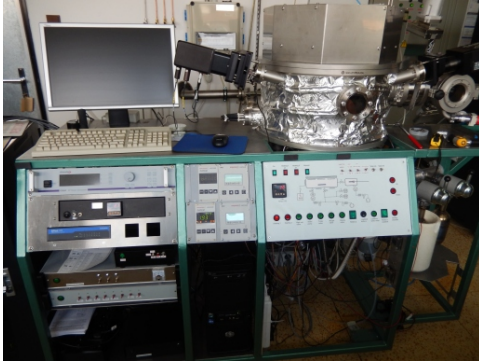
Figure 3.3: Home made magnetron sputtering system
