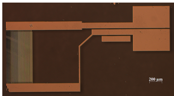
Figure 4.11: Picture of fabricated IDTs using lift-off technique
