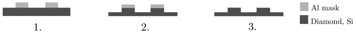
Figure 4.5: Procedure for determination of RIE rate of different materials, 1. Diamond or Si substrate with Al mask, 2. Etched substrate with etched Al mask, 3. Etched substrate after removal of Al mask
