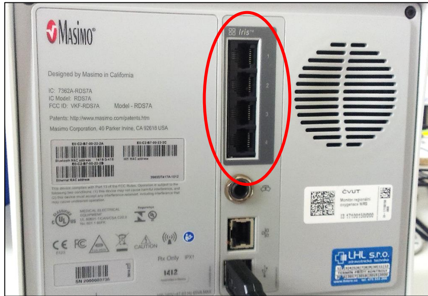
Figure 31. Backside of Masimo’s Root Monitor. Iris™ ports.
