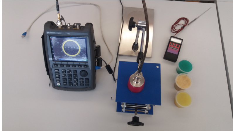
Figure 5: Experimental setup during measurement of dielectric parameters with coaxial dielectric probe and vector network analyzer.
