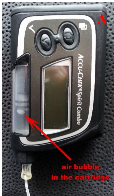
Figure 4: Example of air bubble presented in the infusion set (A) and bent and clogged part of cannula (B).
