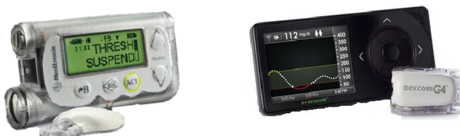
Figure 28: CGM systems used for continuous glucose monitoring of the patients. Left picture – Medtronic MiniMed 530G insulin pump with CGM [84], right picture – Dexcom G4 CGM system [37].
