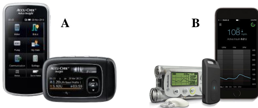
Figure 10: Roche's insulin pump with a data manager for remote control (A) [43] and Medtronic's insulin pump with CGMS sharing data with a smartphone (B) [44].
