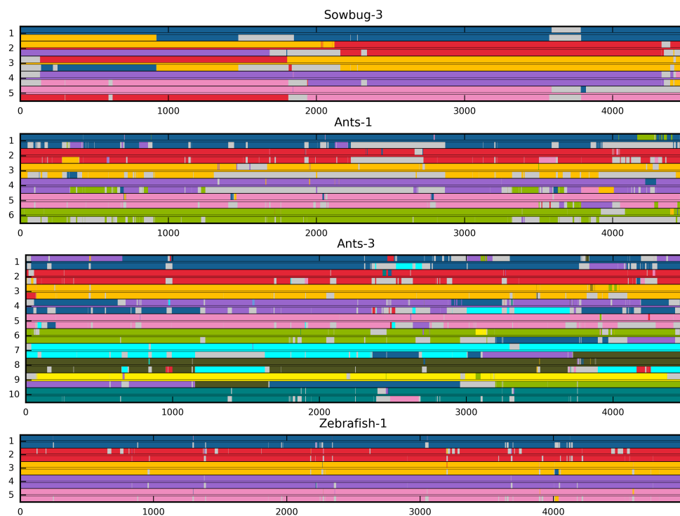
Figure B.1: ID detection results on Sowbug-3, Ants-1, Ants-3, Zebrafish-1 datasets. Y axis labels identities, X axis labels frames. Top row - idTracker (with interpolation), middle (thinner) row - ground truth, bottom row - FERDA (without ID-Consistency Rules and without expert annotations). Gray - ID unassigned.
