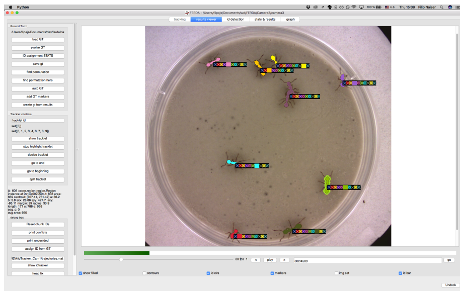
Figure 8.2: A screenshot from FERDA-results-viewer tool. In the middle part, there is a video player with results showed. P and N ID-Sets are visualized by stripes with squares. Where color describes an ID. When it is crossed, it is in N set, when enhanced it is in P set. When segmentation color is dotted it does not represent object ID but tracklet id. Below is the video player and visualization control panel. In the left part, controls for GT creation, other system's results from visualisation and comparison and debugging tool are situated.
