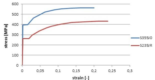
FIGURE 1. Comparison of the working curve of S235JR and S355J0 steel used in simulation [16].
