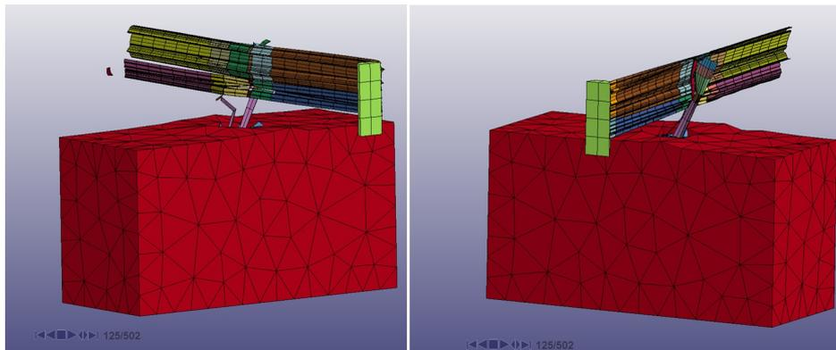
FIGURE 4. Safety barrier deformation at time step 0.125 s — JSAM-2/H2, TB11 [16].
