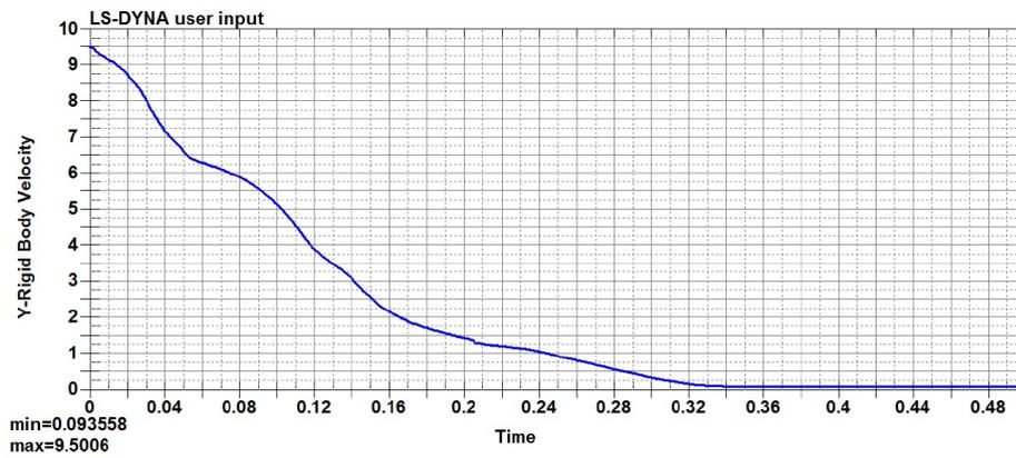
FIGURE 3. Vehicle velocity — JSAM-2/H2, TB11 [16].
