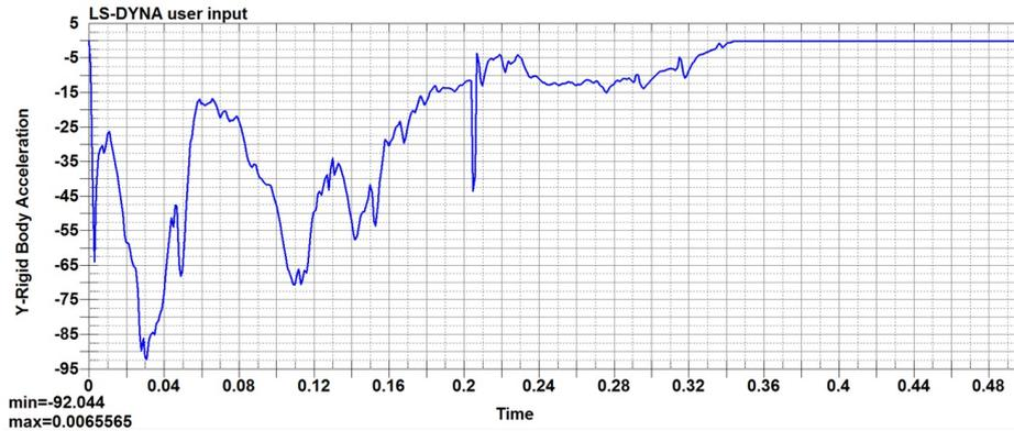
FIGURE 6. Vehicle acceleration — JSAM-2/H2, TB11 [16].
