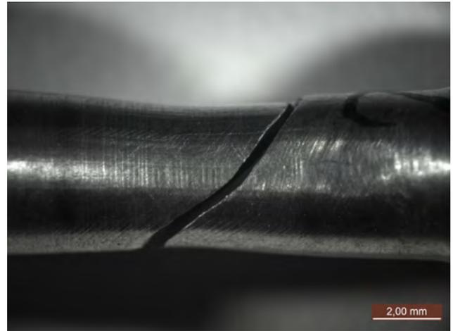
FIGURE 8. Fracture of EN AW 6012 alloy post-ECAP.
