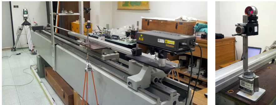
FIGURE 13. Left: Setup of the short periodic test; Right: The interferometer carriage with reflectors.
