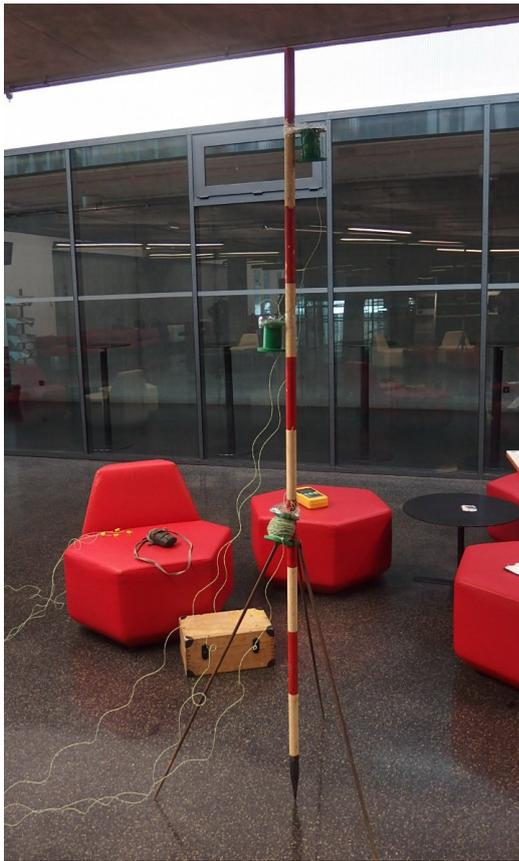
FIGURE 5. Fixing of temperature sensors at the range pole
