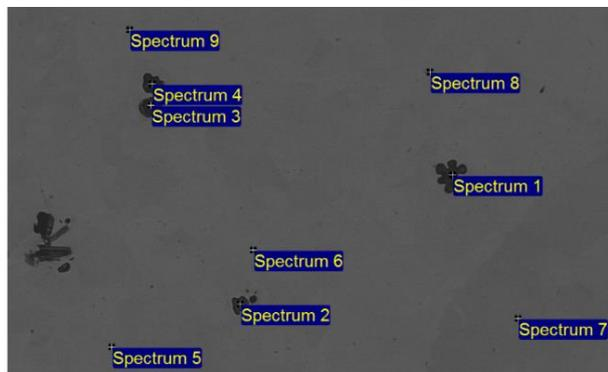
FIGURE 6. Analysed zones of microstructure in Bi2La solder.
