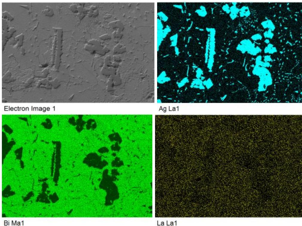
FIGURE 4. Planar analysis of Bi<sub>11</sub>Ag<sub>2</sub>La solder.
