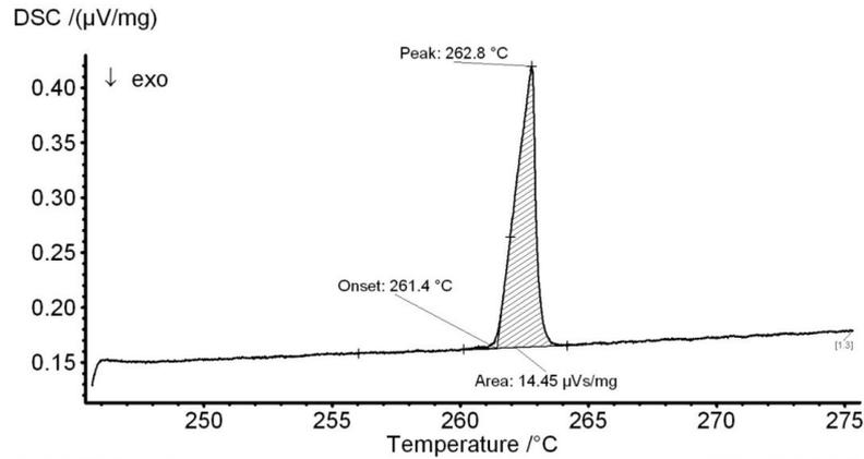
FIGURE 3. DSC analysis of Bi<sub>11</sub>Ag<sub>2</sub>La solder (1 K/min).
