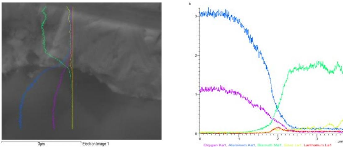
FIGURE 8. Concentration profiles of Bi, La, Ag, Al and O elements on the boundary of Al<sub>2</sub>O<sub>3</sub>/Bi<sub>11</sub>Ag<sub>2</sub>La joint.
