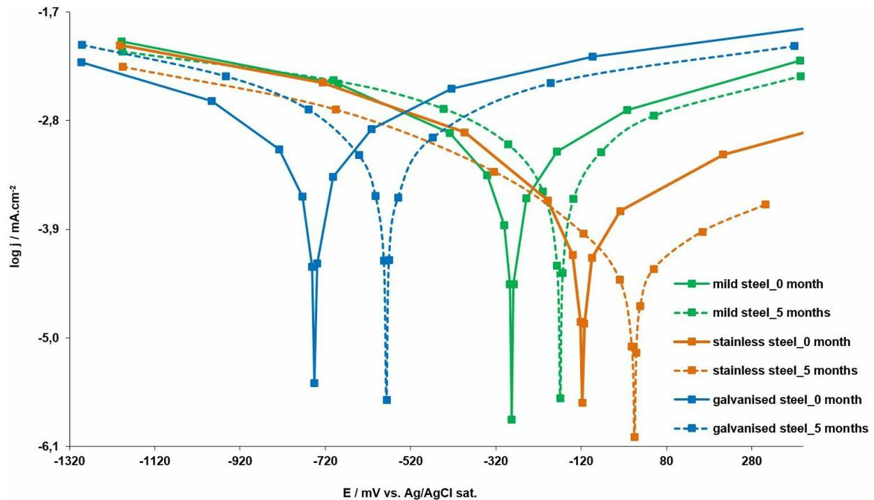
FIGURE 3. Polarization curves of mild, stainless and galvanized steel measured in a layer of artificial rainwater 0.5 mm in thickness; samples before exposure (full line) and after 5 months of exposure (dashed line)
