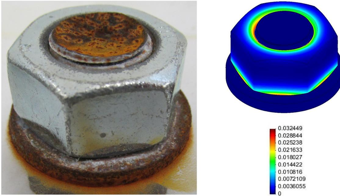
FIGURE 4. Bolt joint 3 after exposure, and the modelled distribution of the corrosion rate [mm/year] during the rainy period
