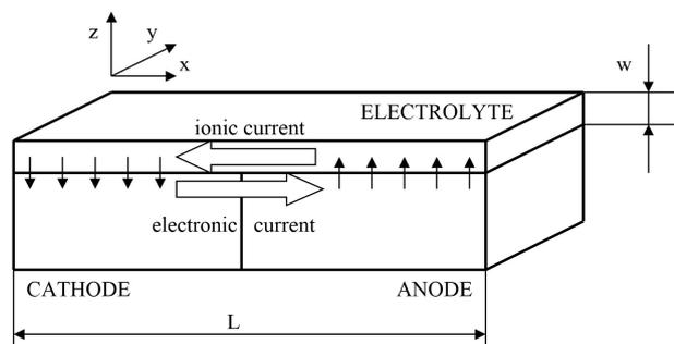
FIGURE 1. Galvanic corrosion under a TEL,  $w \ll L$
