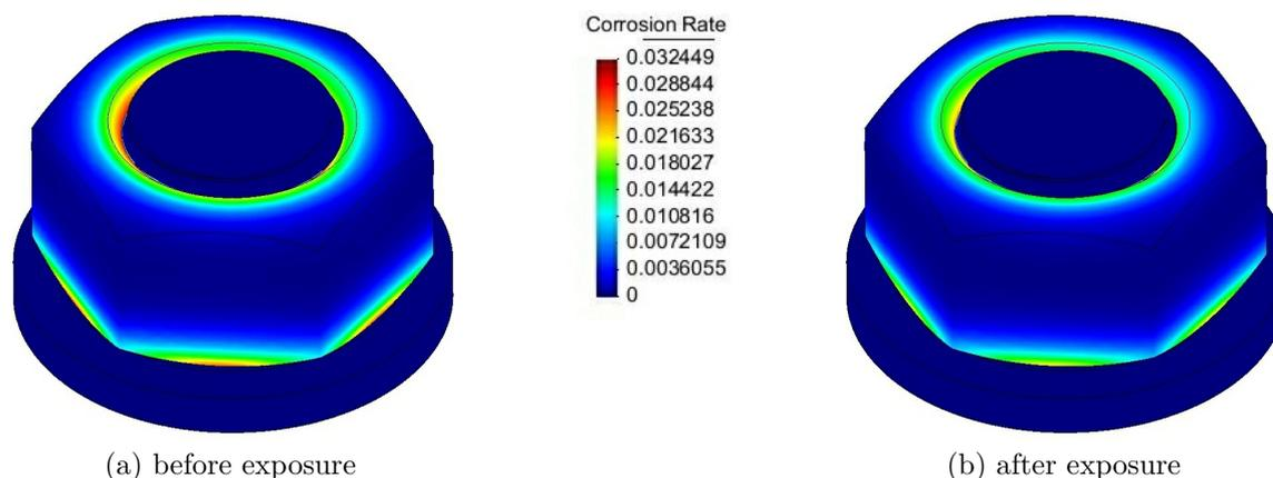
FIGURE 5. Modelled distribution of the corrosion rate [mm/year] on bolt joint 3 during the rainy period using the polarization curves
