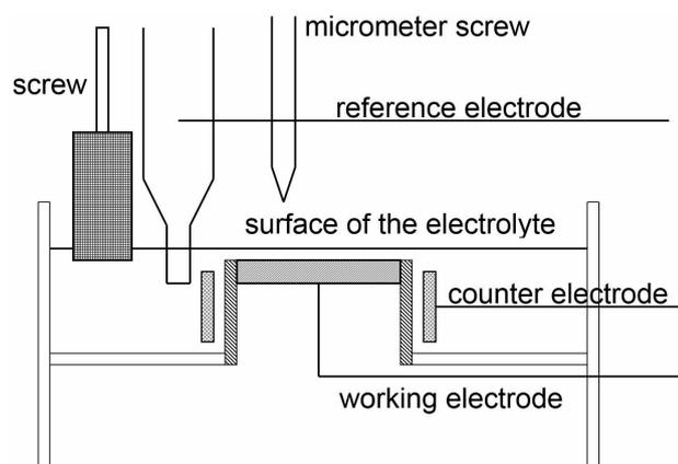
FIGURE 2. Scheme of an electrochemical cell for TEL measurements
