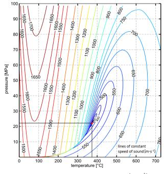
FIGURE 1. Values for the speed of sound  $[m s^{-1}]$  in water and in steam in a p-t diagram.
