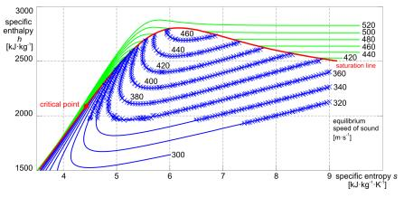
FIGURE 3. The h-s diagram of water and steam with curves of the constant speed of sound in steam  $a \, [m \, s^{-1}]$ . The wet steam region blue lines, are from definition (1) and the blue cross values are calculated by means of the model for normal shock waves. Superheated steam a values according to IAPWS-IF97 are depicted by green curves.
