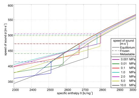
FIGURE 5. Dependence of speed of sound on specific enthalpy for constant pressures.
