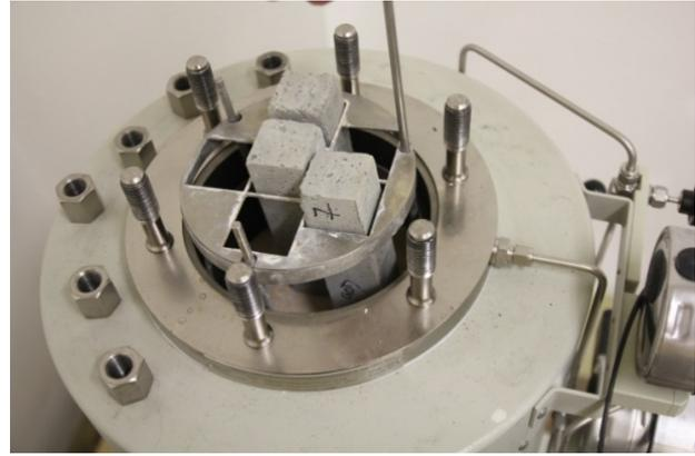
FIGURE 1. Pressure vessel and steel holder with specimens.
