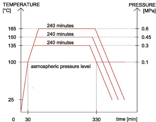
FIGURE 2. Pressure and temperature curves of hydrothermal processes.
