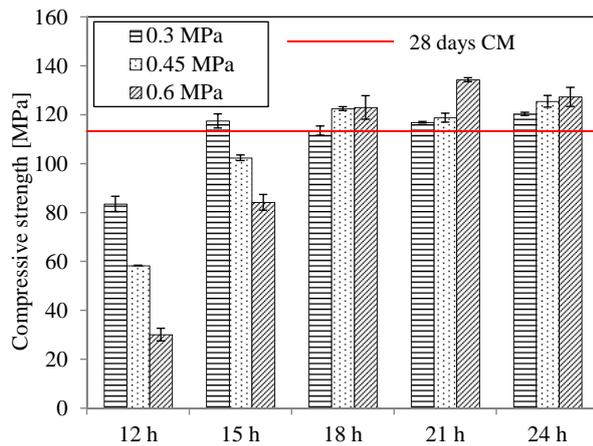
FIGURE 4. Average values of compressive strength  $f_{cm}$  of CM after curing under different conditions.
