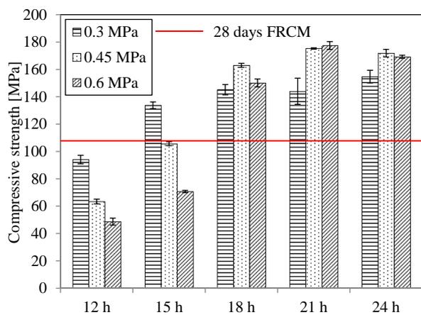
FIGURE 5. Average values of compressive strength  $f_{cm}$  of FRCM after curing under different conditions.
