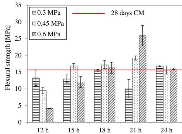
FIGURE 6. Average values of flexural strength  $f_{tm}$  of CM after curing under different conditions.
