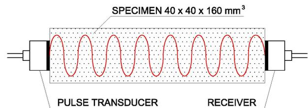
FIGURE 3. Principle of ultrasonic testing.
