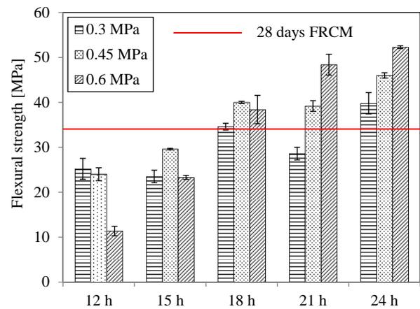
FIGURE 7. Average values of flexural strength  $f_{tm}$  of FRCM after curing under different conditions.
