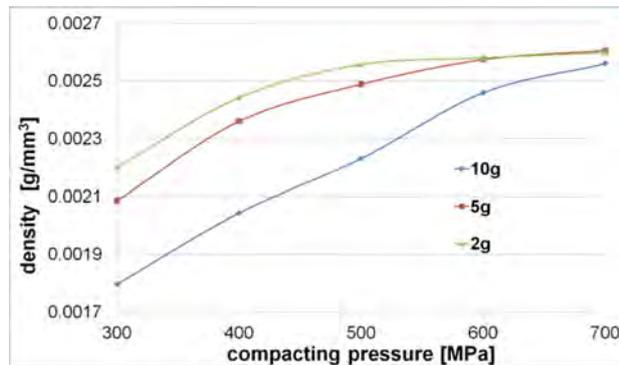
FIGURE 5. Density vs. compacting pressure – the large chips.
