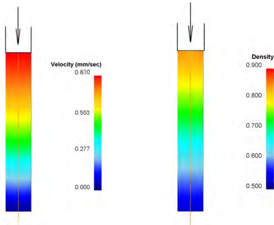
FIGURE 7. Numerical simulation of the compacting process on a 10 g sample under 300 MPa.
