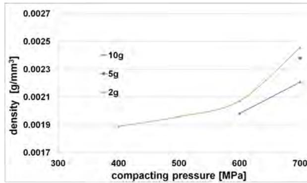
FIGURE 4. Density vs. compacting pressure – the small chips.
