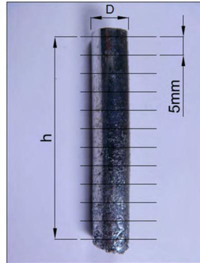
FIGURE 3. Schematic illustration of the division of the sample.
