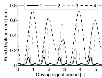
FIGURE 5. Measurement of the displacement versus the time characteristic for four different valve reeds shown in Figure 4. The displacement was measured with the laser beam pointing at the center of the delivery port.
