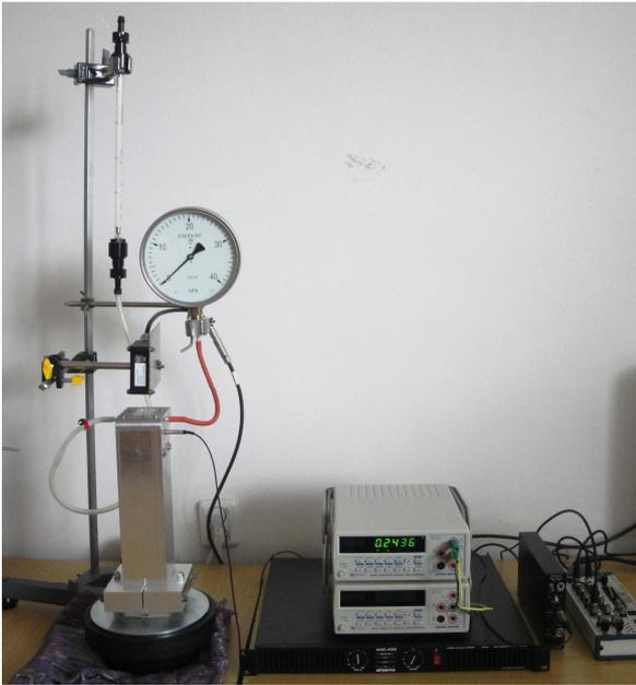
FIGURE 3. The acoustic compressor experimental setup. The selenium driver with the resonator attached to it is in the left part of the picture. The delivery valve housing is attached on the top of the resonator and laser vibrometer is placed above. One of the hoses connects the pressure gauge and the other one with a hose clamp leads to the flow-meter. A microphone is connected from the side of the resonator.
