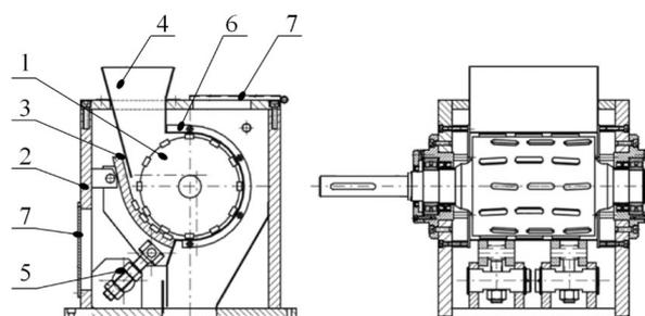
FIGURE 2. Design of a retting mill [19] (1–rotor, 2–cradle, 3–plate, 4–input neck, 5–adjustment screws, 6–drum sieve, 7–control cover).
