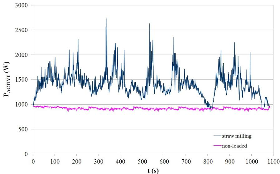
FIGURE 5. A typical measurement record – dependence of total active power over time.
