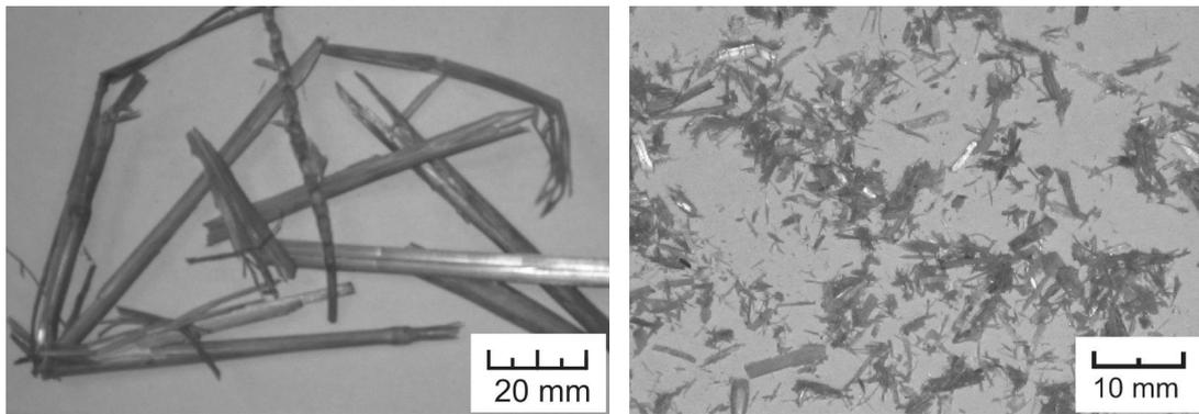
FIGURE 3. Macrostructure of wheat straw: A) before disintegration, B) after disintegration.
