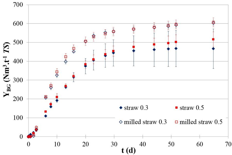
FIGURE 6. Dependence of specific biogas production over time related to TS.
