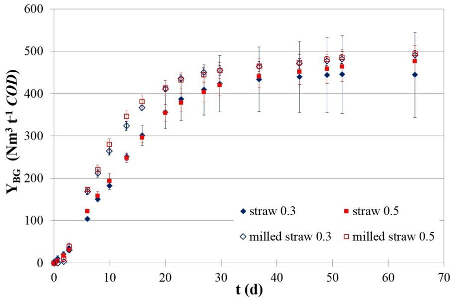
FIGURE 7. Dependence of specific biogas production over time related to COD.
