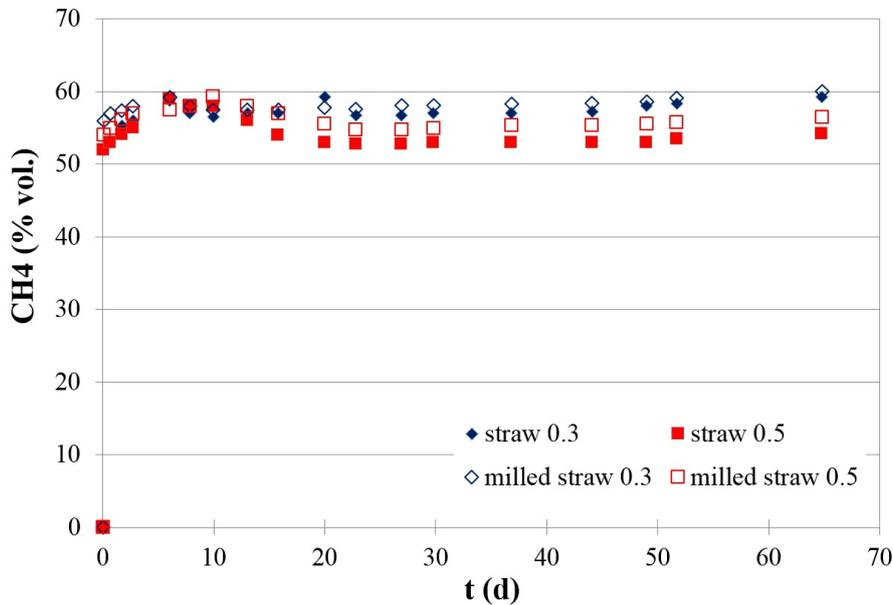
FIGURE 8. Dependence of volumetric methane content in biogas over time.
