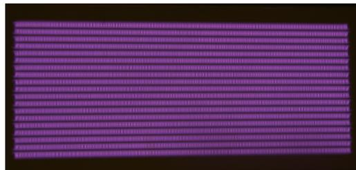
FIGURE 2. Image of DCSBD discharge generated in air at a power input of 400 W. The discharge area is about  $8 \times 20 \text{ cm}^2$ .
