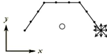
FIGURE 4. The considered shifts of a single point of the two dimensional reflector model used for each step in shape optimization.
