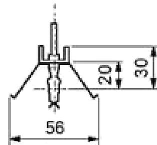
FIGURE 7. A side-view of the reflector used for measurements of the calibration values.
