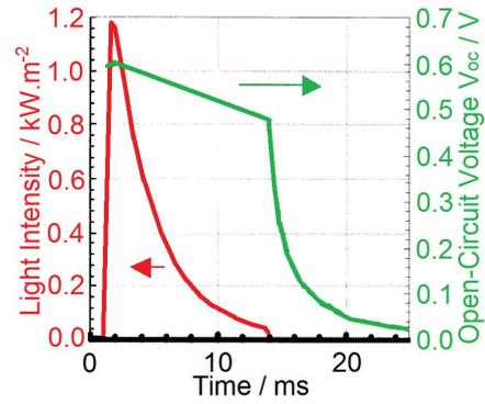
FIGURE 3. Suns- $V_{OC}$  measurement: the decrease in light intensity and the corresponding open-circuit voltage  $V_{OC}$  of the solar cell in time [15].
