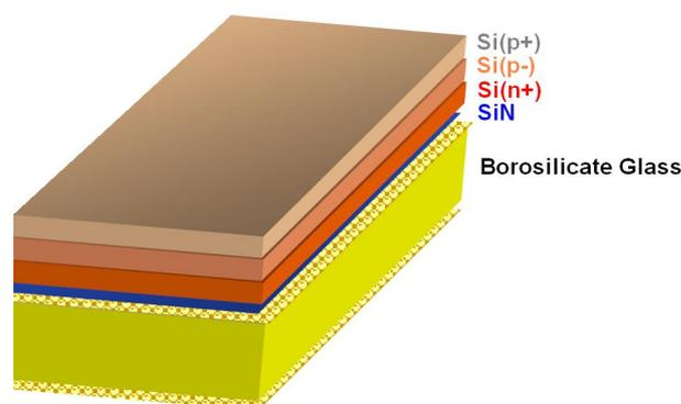
FIGURE 1. Structure of a thin film polycrystalline silicon solar cell fabricated by CSG Solar AG without metallization to allow passivation in water vapour [9].
