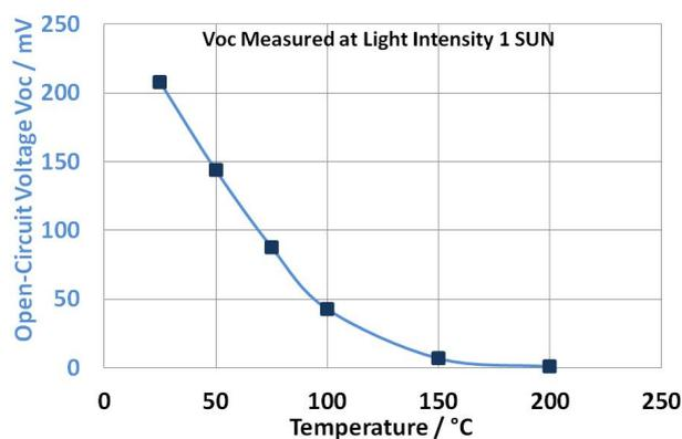
FIGURE 6. Temperature dependence of open-circuit voltage  $V_{OC}$  for a tested non-passivated thin film polycrystalline silicon solar cell.
