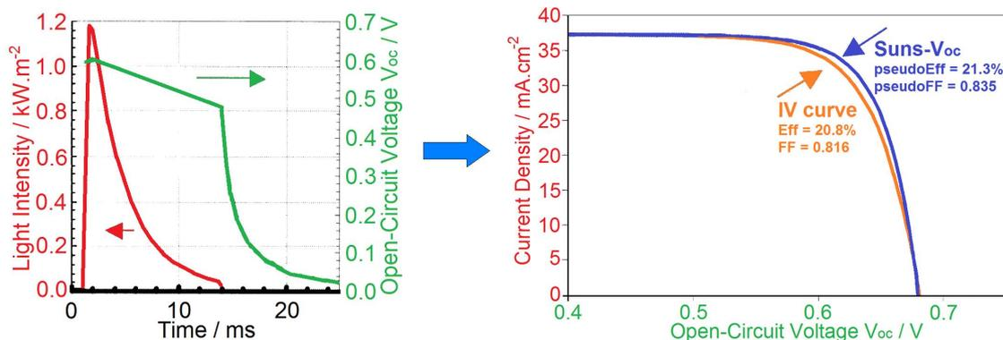
FIGURE 5. Creation of a Suns- $V_{OC}$  current-voltage characteristic from the measured light intensity and the corresponding  $V_{OC}$ . Comparison of a Suns- $V_{OC}$  measurement with a current-voltage characteristic of the same solar cell measured in the common way [15].
