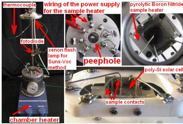
FIGURE 2. Apparatus comprising the stainless steel pressure chamber, the heater, the xenon flash lamp, the thermocouple, the pyrolytic Boron Nitride sample heater, and stainless steel probes to contact the investigated thin film poly-Si solar cell used for investigating water vapour passivation.
