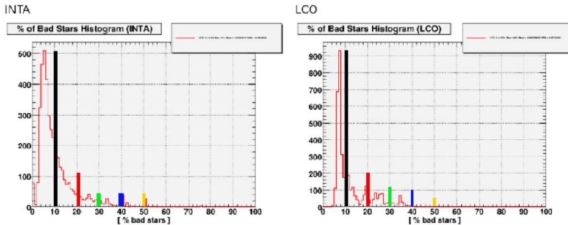
FIGURE 6. Histograms of the percentage of bad catalog stars in a single frame. These histograms were created for a given range of frames, and for each frame it was calculated what percentage of catalog stars from the analyzed frame have  $|M_{\text{corr}} - \text{Med}| > 2\sigma$ . We assumed that the best frames have less than 10% bad catalog stars and the worst frames have more than 50% bad catalog stars.
