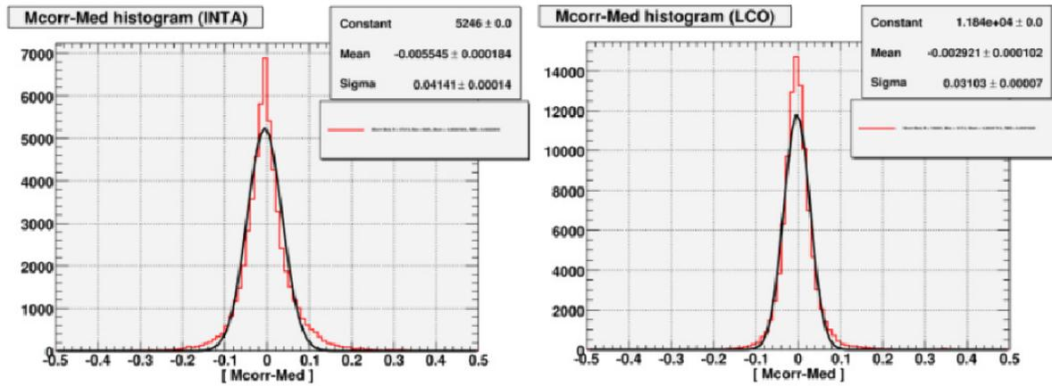
FIGURE 5. The Gauss function fitted to  $|M_{\text{corr}} - \text{Med}|$  histogram. Thanks to this fit we can obtain the value of  $\sigma$ , which is later used to calculate the quality of the analyzed frames.
