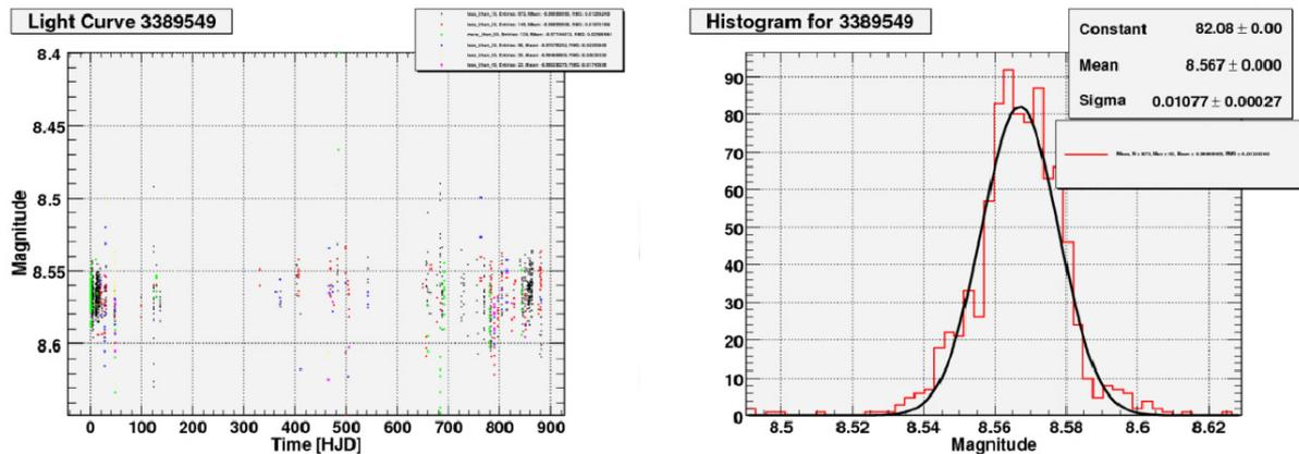
FIGURE 8. The light curve of an analyzed star after using the statistical data quality estimate method (on the left). Colors represents the quality of the analyzed measurements. A histogram of this light curve after removing all bad data (on the right). As we see, after using this method the light curve quality improves significantly and  $\sigma \sim 0.01^m$  is achieved.
