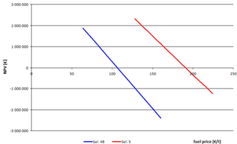
FIGURE 4. Chart showing the dependence of NPV on fuel price.
