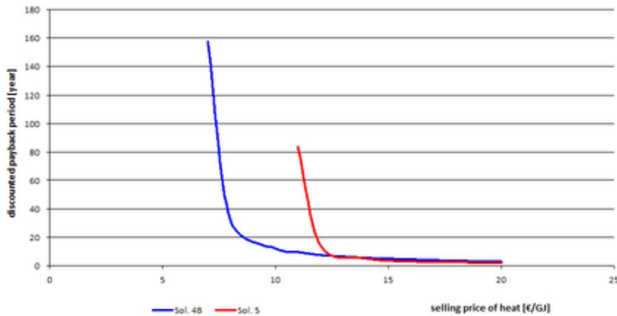
FIGURE 7. Chart showing the dependence of the discounted payback period on the selling price of heat.
