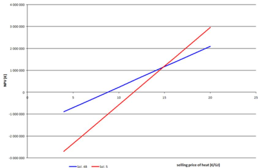
FIGURE 6. Chart showing the dependence of NPV on the selling price of heat.
