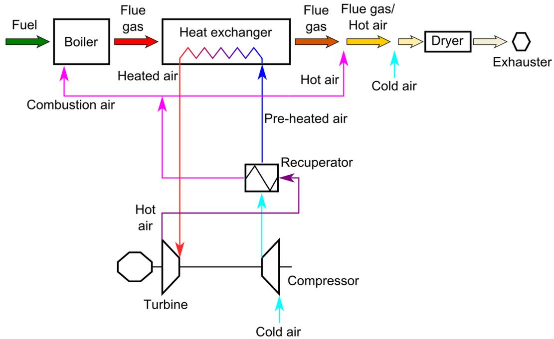
FIGURE 1. Scheme of the designed technology — Solution 1.
