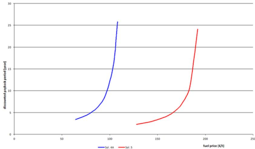
FIGURE 5. Chart showing the dependence of the discounted payback period on fuel price.
