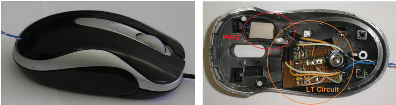
FIGURE 4. Implementation of the PVF2 piezomaterial on the left mouse button and the LT EH circuit.
