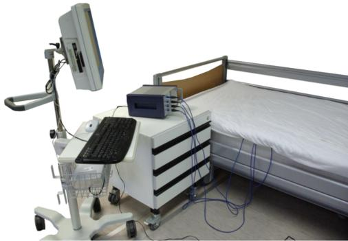
FIGURE 1. Sensor-system setup in a bed.
