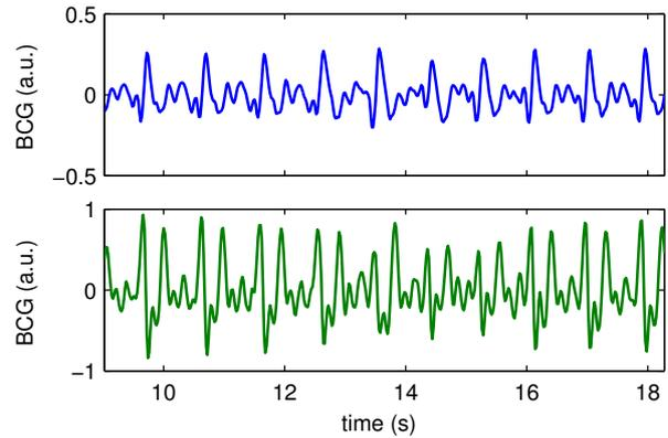
FIGURE 6. 2-channel BCG data (0.5–20 Hz)-filtered BCG Signal.
