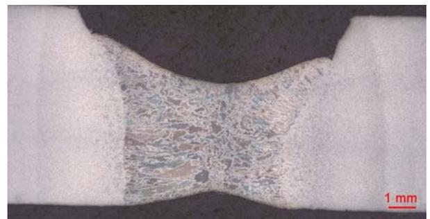
Figure 6: Sample B3 — root weld, short arc 130 A
