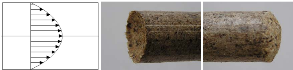
Figure 6: Pressing force distribution across the pressing chamber
