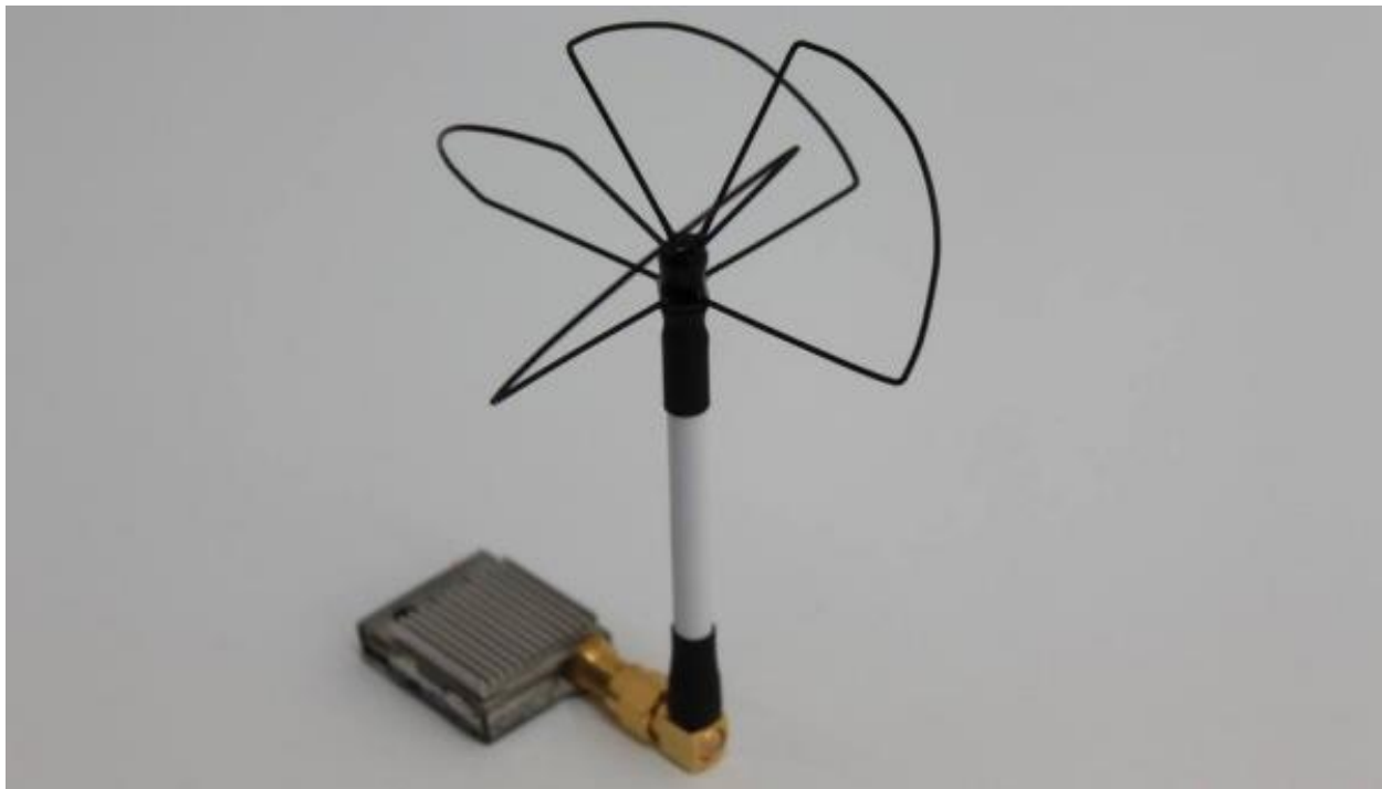
Obr. 6 - Skew Antenna Planar Wheel [3]
